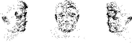
Figure 3. Sparse set of 3d points after using a structure-from-motion algorithm on the sequence of Fig. 2. From left to right, the 3d points are shown from three different viewpoints roughly at -45 degrees, 0 degrees, and 45 degrees.
