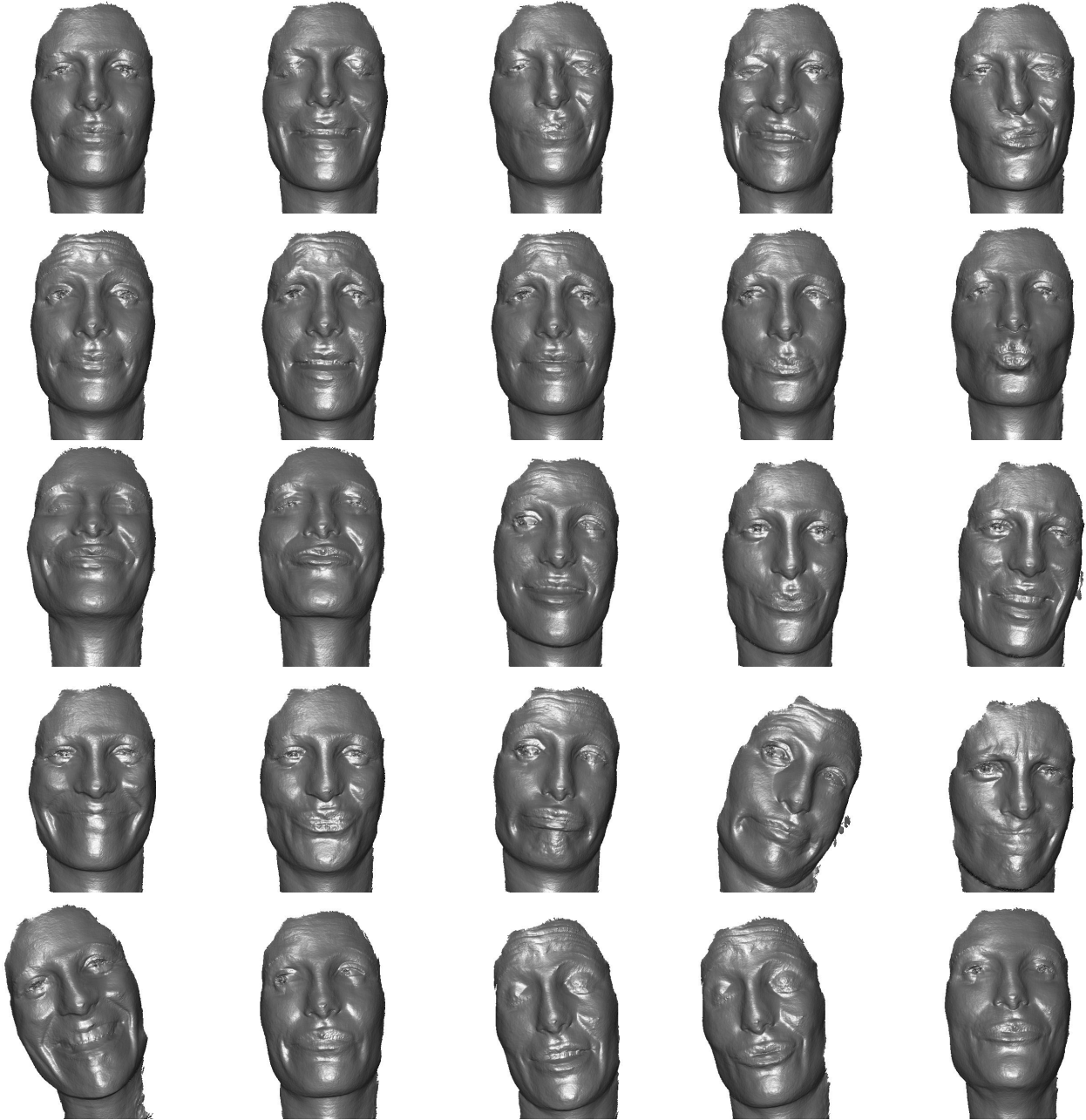
Figure 12. Acquisition of 3d facial expressions using [10]. The system was calibrated using the self-calibration technique described in this paper.
