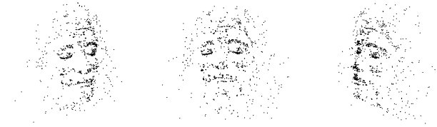
Figure 8. Sparse set of 3d points after using a structure-from-motion algorithm on the sequence of Fig. 7. From left to right, the 3d points are shown from three different viewpoints roughly at -45 degrees, 0 degrees, and 45 degrees.
