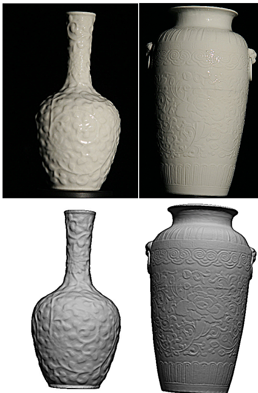
Figure 2: Reconstructing porcelain vases. Top: sample of input images. Bottom: proposed method. The resulting surface captures all the fine details present in the images, even in the presence of strong highlights.
