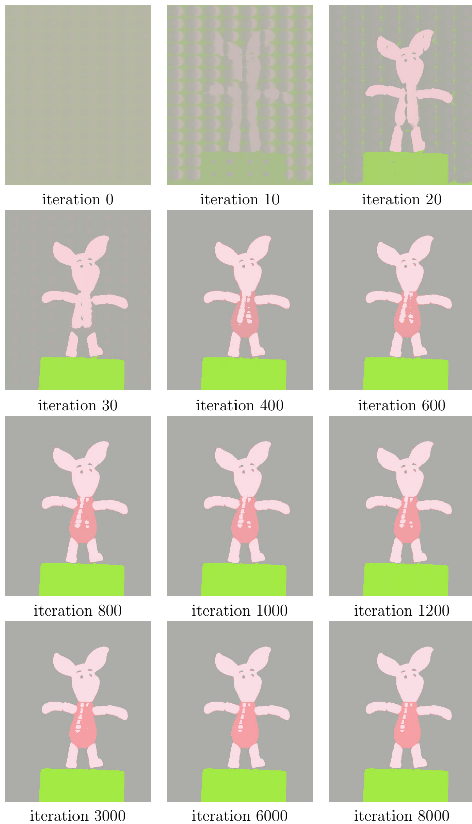
Figure A.11: 4-phase segmentation using [Vese and Chan, 2002] speed. The level sets are able to converge to the global minimum. The four regions are drawn with their corresponding mean color.
