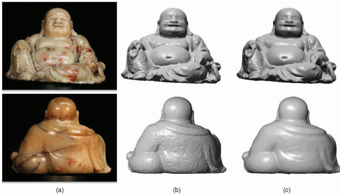
Fig. 7. Reconstructing colored jade. (a) Two input images. (b) Model obtained by multiview stereo method from [16]. (c) Proposed method. The resulting surface is filtered from noise, while new high frequency geometry is revealed (note the reconstructed surface cracks in the middle of the figurine's back).
