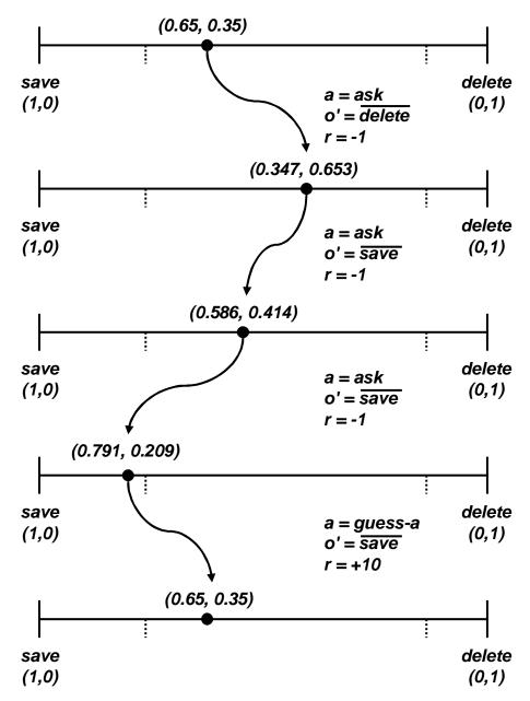
Figure 4: Evolution of the belief state in the example voicemail spoken dialog system POMDP. The dashed lines show the partition policy, given in Figure 3. At each time-step, the point *b* is updated using equation (2). Note that a recognition error is made after the first "ask" action.
