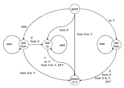
Figure 19: *HC1* handcrafted policy represented as a finite state controller. Node labels show the POMDP action to take for each node, and arcs show which POMDP observations cause which transitions. Note that the nodes in the diagram are entirely indepenent of the POMDP states.
