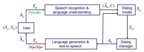
Figure 5: Typical architecture of a spoken dialog system
