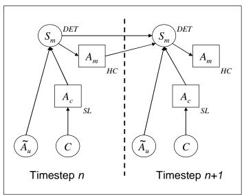
Figure 9: Influence diagram showing how a confidence score is typically incorporated into a spoken dialog system. Node C is a random variable representing confidence score.  $A_c$  may take on values such as  $\{hi, low\}, \{explicit-confirm, implicit-confirm, reject\}, etc.$
