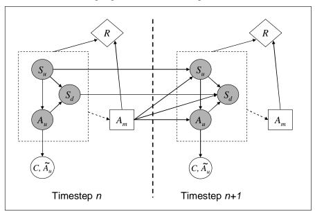
Figure 6: Influence diagram representation of the SDS-POMDP model. The dashed box indicates the composite state s which is comprised of three components,  $s_u$ ,  $s_d$ , and  $a_u$  (see text for a complete definition of variables). The dashed line from the dashed box to  $a_m$  indicates that the action  $a_m$  is a function of the belief state  $s_m = b(s_u, a_u, s_d)$ .
