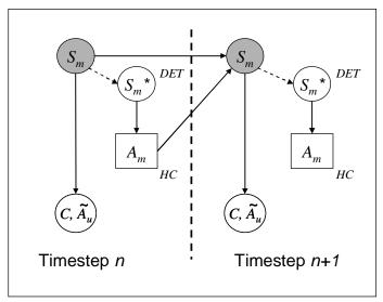
Figure 8: Influence diagram showing multiple state hypotheses.  $S_m^*$  takes the value of the state  $S_m$  with the highest probability mass at each time-step. The superscript DET indicates that the variable  $S_m^*$  is not random but is rather a *deterministic* function of its inputs.
