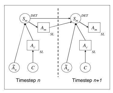
Figure 10: Supervised learning for action selection. The node  $A_m$  has been trained using supervised learning on a corpus of dialogs (indicated with the SL subscript). The DET superscript on  $S_m$  indicates that this node is deterministic.
