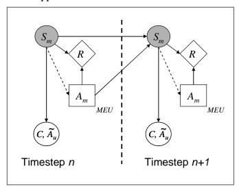
Figure 7: View of a spoken dialog system as a greedy decision theoretic process. Action  $A_m$  is selected to maximize the expected immediately utility R, indicated by the subscript MEU ("Maximum Expected Utility"). The dashed line indicates that  $A_m$  is a function of the distribution over  $S_m$ , rather than its actual (unobserved) value.
