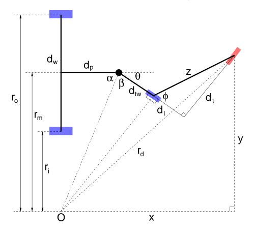
The geometrical properties of the domino laying vehicle are shown in the diagram above. The drive and trolley wheels are drawn in blue, with the deposited domino in red. Our aim is to lay the dominoes in a circle of radius  $r_d$  around the origin O. To do this, we need to find the radii  $r_i$  and  $r_o$  traced out by the inner and outer drive wheels. We can then set the speeds of the two drive motors according to the ratio  $r_i/r_o$ .
