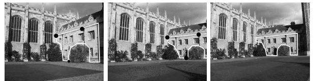
Figure 9: A surface is added to the model by specifying it in one view. Three points must be matched to define the plane. The segment can be projected into all of the images.
