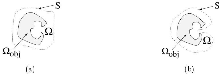
Figure 2: (a) Example of a shape which cannot be reconstructed, (b) alternative choice for S that allows the cavity to be reconstructed.
