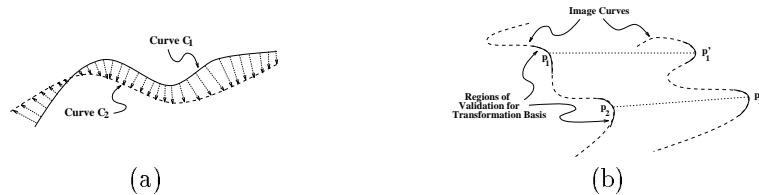
Fig. 2. (a) The deviation of C_1 to C_2 is the integral of squared distances from points on C_1 perpendicular to C_2 , as defined by definition 2. (b) A neighbourhood-validated basis comprising of 2 correspondences is shown.
