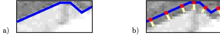
Fig. 2. Edge tracking example. (a) Edge in initial frame. (b) In the next frame the image edge has moved. Tracking nodes are initialised along the model edge and then search normal to the edge to find the new location. The best-fit motion is the one that minimises the squared distance error between the tracking nodes and the edge.
