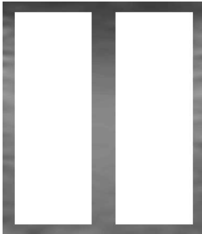
Figure 8: Regions used to calculate SNR estimates. Within a single frame, the two regions indicated by white boxes were used to calculate two estimates of SNR. They are separated laterally and leave a gap at the edges to allow for the filter capturing values outside these regions. Within each simulated data set, five frames like this were used to obtain ten estimates of SNR.
