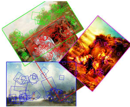
Figure 1: Sample Retrieval Result . This is a sample query image, in which reference images from the database have been artificially modified and made to occlude each other to test retrieval in difficult situations. The rectangles around each image indicate that it has been correctly identified, with the smaller rectangles within each indicating what features were used in the matching process.
