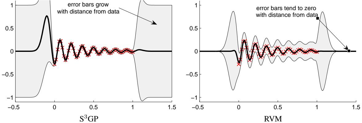
Figure 6. Gaussian process error bars. In this synthetic one-dimensional example, the  $S^3\text{GP}$  is compared to the RVM [15]. Crosses indicate training data points for which an appropriate dynamical prior is known and the solid lines are the mean interpolants which, for both cases, are good. The shaded region shows the 90% confidence interval and it can be seen that the  $S^3\text{GP}$  is subjectively better in that it becomes *less* confident as distance from the training data increases.
