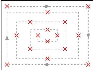
Figure 3. Gaze calibration pattern. An animated target moves around the screen in a spiral pattern. At 16 *milestones* (marked “x” in diagram) the target comes to rest for 1 second and a labelled exemplar is recorded. As the point moves between each milestone, 5 further unlabelled exemplars are also recorded. See additional material.
