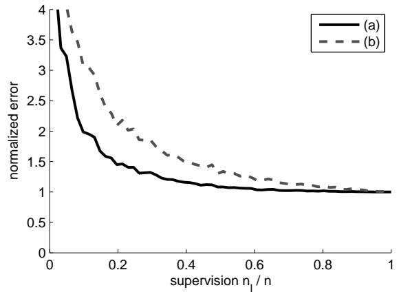
Figure 8. Semi-supervised performance. This graph shows the variation of  $S^3\text{GP}$  accuracy with supervision: the error has been normalized such that the supervised ( $n_l = n$ ) solution has an error of 1. (a)  $S^3\text{GP}$  performance on eye data. (b) Gaussian process performance ignoring unlabelled exemplars.
