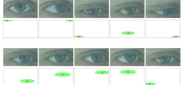
Figure 1. Inferring gaze with the  $S^3GP$ . This figure shows closeup eye images (mirrored around the vertical axis), and the correspondingly inferred gaze position on the screen. The ellipse indicates the  $\pm 2$  standard deviation error bars in the prediction. This video may be seen in the additional submitted material.
