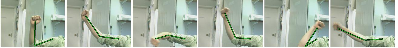
Figure 11. Mapping to higher dimensions. In this example, the S<sup>3</sup>GP has learnt the mapping from images to 2D hand/elbow position, resulting in a four-dimensional output space. Once trained, pose inference takes place in real-time, requiring 55% CPU cycles. This is shown in the video included as additional material.
