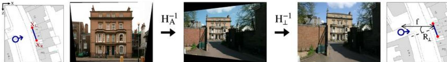
Rectifying rotation  $R_{\perp}$  gives the angle from perpendicular and focal length the distance to camera.
