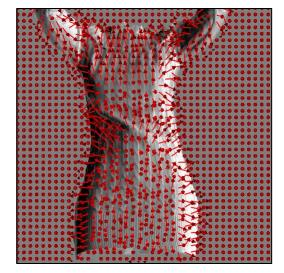
RGB Color is converted to a normal at each pixel
