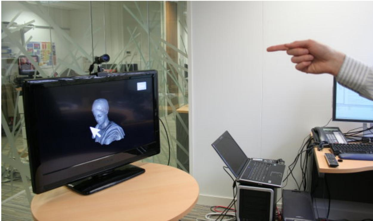
Pointing around the screen moves the viewing angle of the object
