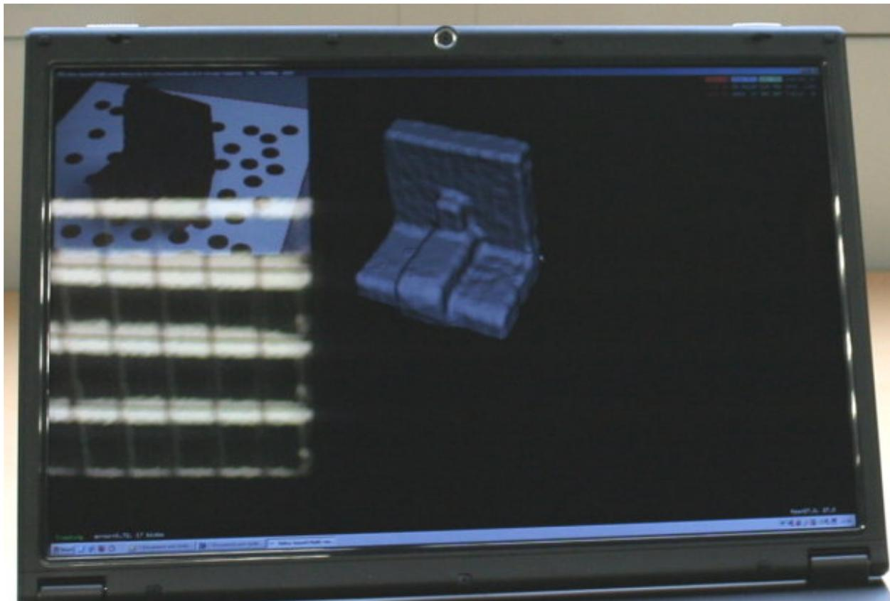
The polystyrene object (shown above) digitally recreated with a complete surface but without texture mapping
