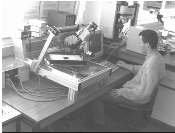
Figure 10: The IRVIS system for circuit board inspection in use
