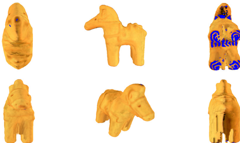
Fig. 10. 3D model of the Haniwa built from the estimated circular motion alone. The gaps between the legs were not carved away since they never appeared as part of the profiles, and textures were missing in areas (top and bottom) which were invisible under circular motion.
