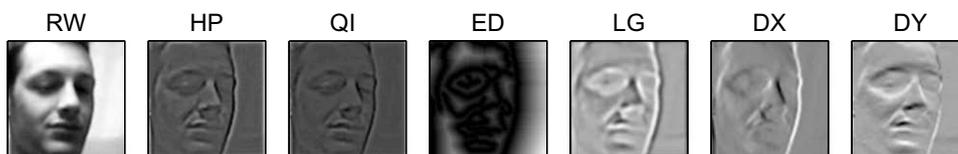
**Fig. 12.** Examples of the evaluated face representations: raw greyscale input (RW), high-pass-filtered data (HP), the Quotient Image (QI), distance-transformed edge map (ED), Laplacian-of-Gaussian-filtered data (LG) and the two principal axis derivatives (DX and DY).
