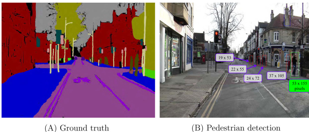
Fig. 10. (A) Human-labeled pseudocolor image showing classes visible in frame 1800 of seq05VD. (B) Example result image from testing our implementation of the Dalal and Triggs pedestrian detection algorithm (Dalal and Triggs, 2005) on our database. People who appear as size 64 \times 128 pixels or larger are usually detected (shown as green boxes). People smaller than that in image-space are often not detected (shown as red rectangles). In contrast to the INRIA database, the CamVid Database has no images of people posing, so they appear here naturally as they would to a car or CCTV. (For interpretation of the references in color in this figure legend, the reader is referred to the web version of this article.)
