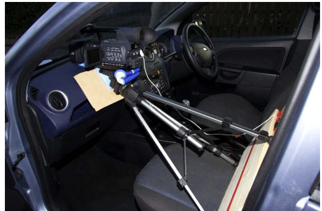
Fig. 2. High-definition camera mounted on the dashboard.
