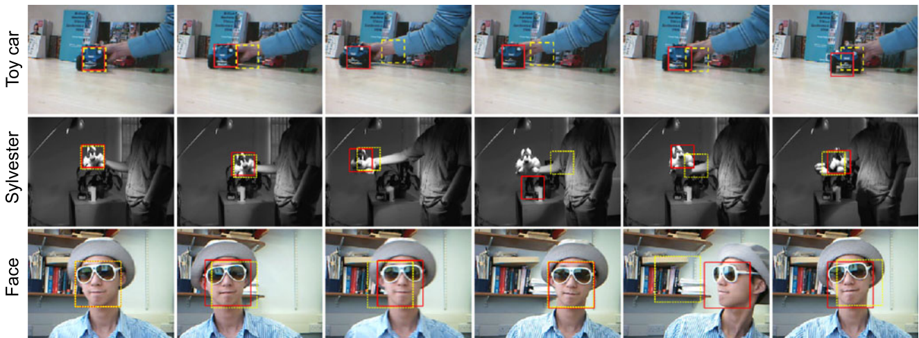
Fig. 11 (Color online) Performance of Boosting and Super tree trackers. Super tree tracker ( solid red line ) achieves a better tracking accuracy by faster classification than Boosting tracker ( dashed yellow line ).
