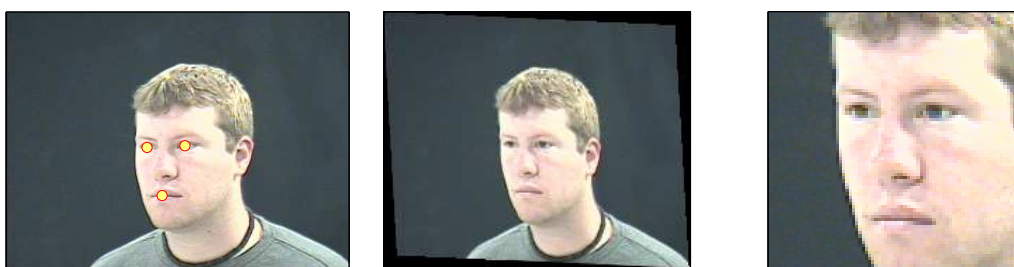
Fig. 3. Registration: Shown is the original image in the visual spectrum with detected facial features marked by yellow circles (left), the result of affine warping the image to the canonical frame (centre) and the final registered and cropped facial image.
