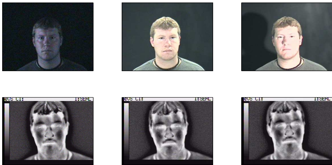
Fig. 1. Sensitivity to lighting conditions: Illumination changes have a dramatic effect on images acquired in the visible light spectrum (top row). In contrast, thermal imagery (bottom row) shows remarkable invariance.
