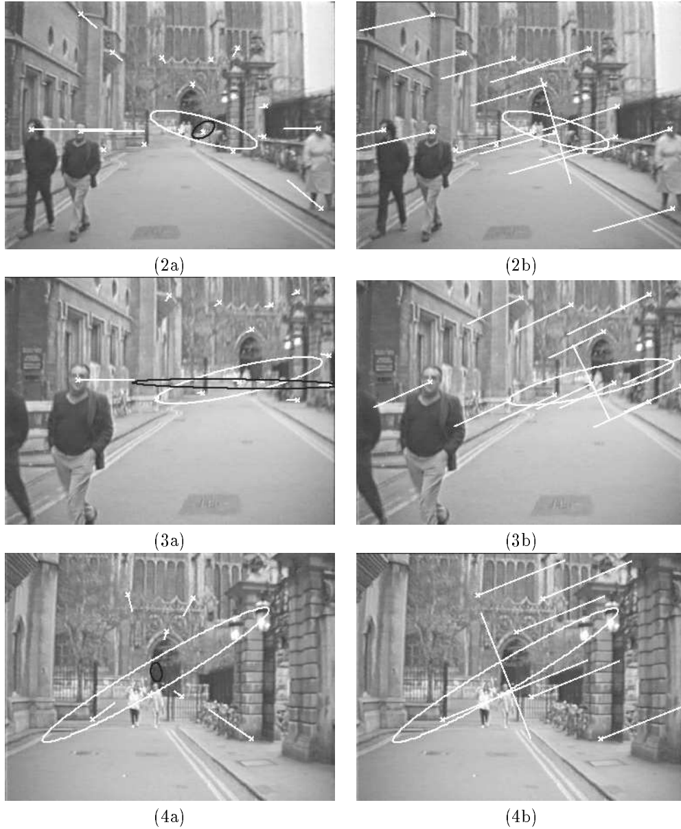
Figure 8: The approach to Kings College Chapel North Gate (Frames 1–4) using Affine Motion Parallax, showing the epipole and extracted translational components (a) and the extracted rotation axis and rotational components (b) (as in figure 5). Again the translational component magnitudes appear as expected (see Equation 3) and are all in the direction of the epipole. The people move in the image as stationary objects twice as close would, and therefore are not rejected as independent motion.
