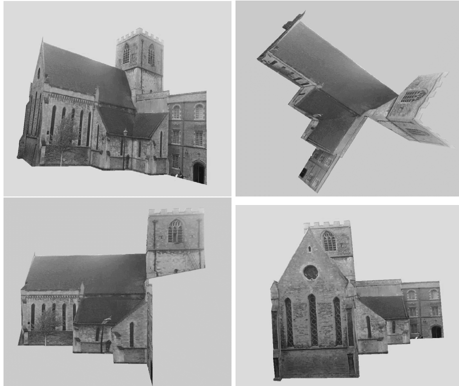
Figure 4: The 3D model can be output in VRML format and viewed from new viewpoints. Four novel views are shown of the reconstructed model. The texture is automatically extracted from the pair of original uncalibrated photographs.
