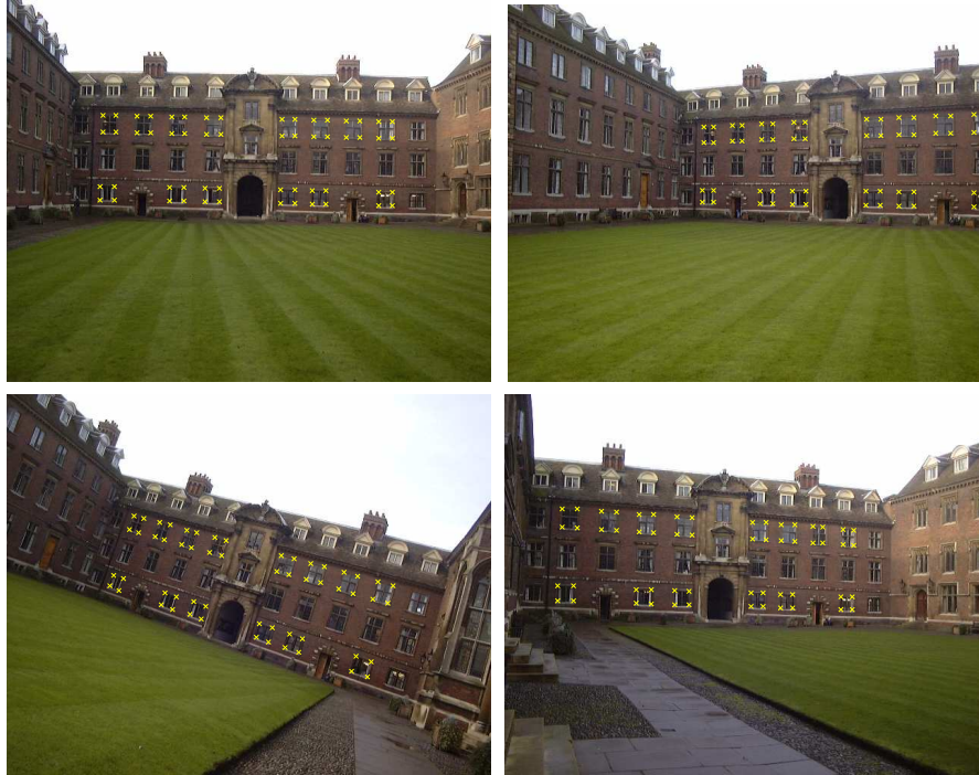
Fig. 4. Four images of a facade. The corners of the windows (marked with a white cross) belong roughly to a plane. They are used to compute the super-collineation matrix from which it is possible to self-calibrate the camera.
