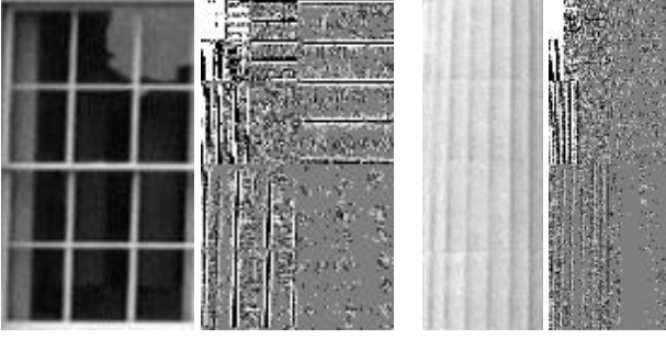
Figure 3. Window and column texture. Beside each texture is its corresponding (quantised) wavelet transform. Output is shown for 3 levels of the wavelet transform. At each level, the HL (horizontal high-pass, vertical low-pass) component is shown at the bottom left, the HH component at the bottom right, the LH component at the top right and the LL component at the top left. The HL component responds strongly to vertical edges, while the LH component detects horizontal edges. The LL component is a smoothed, subsampled version of the original texture.
