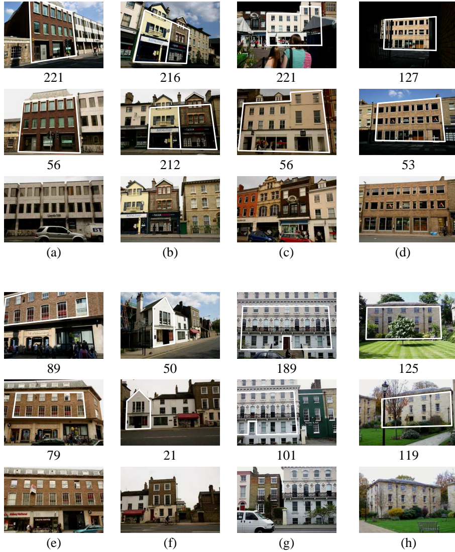
Figure 3: Illustrative database retrieval results. The first rows show query views. The second and third rows show the best and second best database retrieval results together with the number of robustly estimated correspondences. The first six images (a-f) show correct database retrieval results. Transferred building outlines demonstrate the accuracy of the recovered pose estimates. In (g), the correct database view has been recovered but the scale-plus-translation transformation is wrong. In (h), the wrong view has been retrieved because the two buildings are identical.
