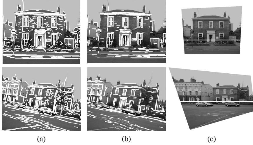
Figure 1: Obtaining canonical views. (a) Straight line segments are detected in left and right views and dominant vanishing points are recovered automatically. Line segments associated with the horizontal and vertical vanishing points are shown in (b). Finally, the images are transformed into a canonical frame corresponding to a rectified view of the dominant plane (c). In the rectified views, the horizon line is horizontal.
