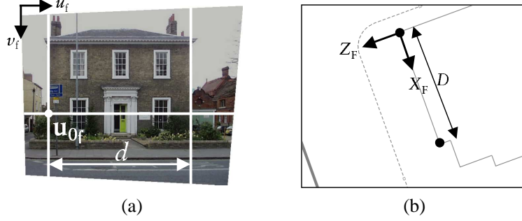
Figure 2: Building facades in the database are associated with a meaningful coordinate system using a map. (a) Two vertical lines are identified manually in each database view (the horizon line is also shown). (b) These lines correspond to points on the map (circles). The point u_{0f} is the projection of origin of the facade coordinate system X_F Y_F Z_F .
