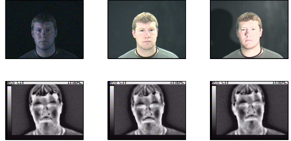
Figure 1: Invariance: Illumination changes have a dramatic effects on images acquired in the visible light spectrum (top row). In contrast, thermal imagery (bottom row) shows remarkable invariance.
