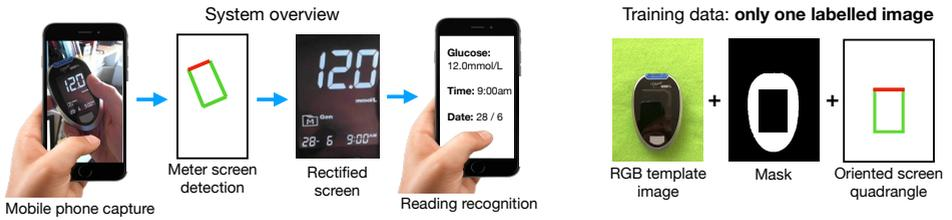
Figure 1: **Real-time screen reading on mobile phone.** Our system can be trained to read a digital meter screen at near 100% read accuracy for in-the-wild conditions. The system can be trained using only one human labelled image consisting of a binary mask indicating screen and background pixels, and the four corner coordinates of the screen.
