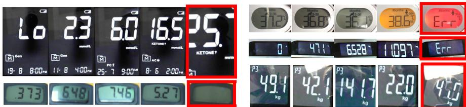
Figure 5: **Digit-recognition dataset**. 5 example screen snapshots from each of our digital meters is shown. First four columns are *valid* examples with the last column an *invalid* example (marked with red border). Notice the difficulty in recognizing the digits due to lighting and reflections.
