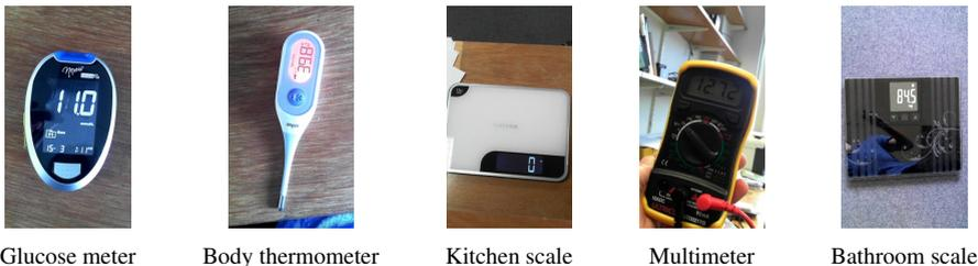
Figure 4: **Digital meters** used in our *Screen-detection* dataset. Screen reflection on these glossy displays severely inhibits screen detection and digit recognition.
