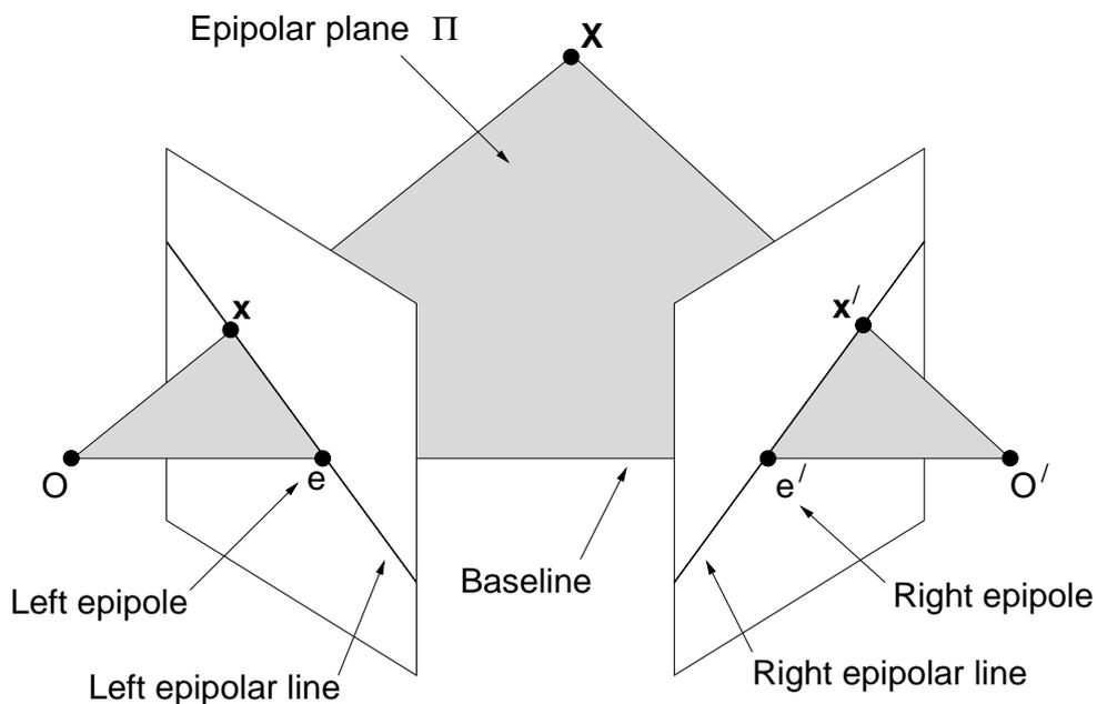
The **epipolar plane** is the plane defined by a 3D point  $\mathbf{X}$  and the optical centres.
