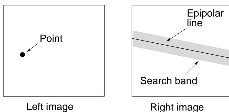
Using the epipolar and other constraints (ordering etc.), we obtain a large number of matches.
