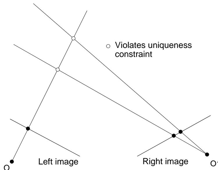
For transparent objects, we cannot rely on the uniqueness constraint. Two features may be visible in the right image but instantaneously aligned in the left image.
