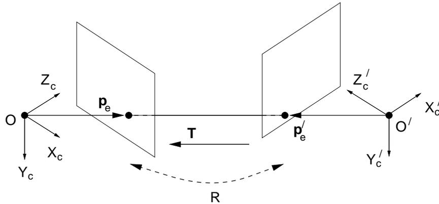
Referring to the figure, the position of the left camera's epipole is  $\mathbf{p}_e$  in the left camera's coordinate system and  $\lambda\mathbf{T}$  in the right camera's coordinate system. Relating the coordinate systems, we obtain
