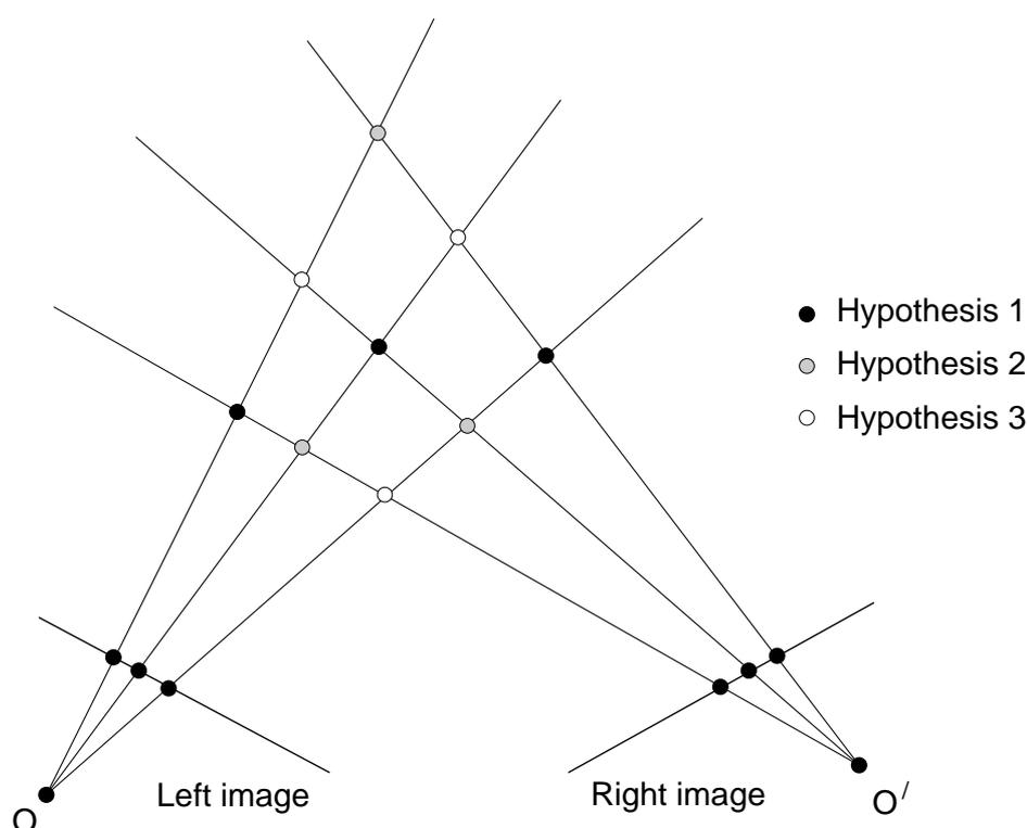
In the illustration, we are trying to match three corners in the left image with three corners in the right image. We have three hypotheses, all of which satisfy the epipolar constraint. How can we discover which hypothesis is correct?
