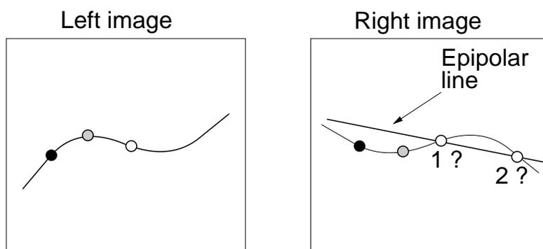
Given matches ● and ○, point ○ in the left image must match point 1 in the right image. Point 2 would exceed the disparity gradient limit.
