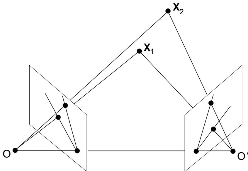
For different world points  $\mathbf{X}$ , the epipolar plane rotates about the baseline. All epipolar lines intersect at the epipole.
