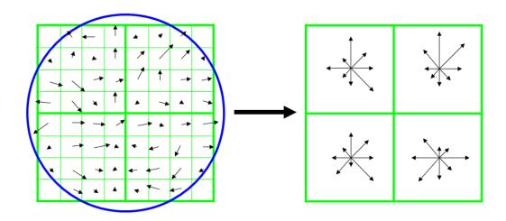
The SIFT (Scale-Invariant Feature Transform) descriptor is an orientation histogram-based descriptor, and is based upon describing the edges in the neighborhood of an interest point in a way which is robust to translation, rotation and scale.
