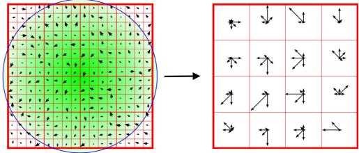
The  $N \times N$  patch is split into c cells, and within each cell the intensity gradient at every pixel is calculated and the directions binned into a histogram weighted by their magnitude and a Gaussian window with a  $\sigma$  of .5 times the scale of the feature centered on the patch. This weights the inner pixels (those closer to the interest point) to avoid possible occlusion problems.
