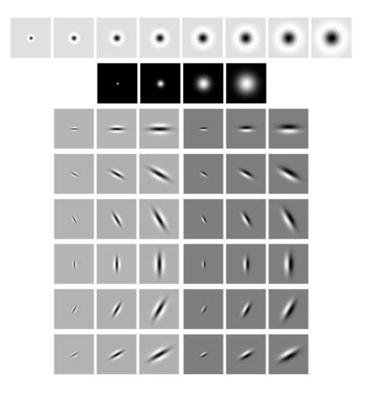
This is an example filter bank. It consists of 8 Laplacian of Gaussian filters and 4 Gaussian filters at different scales to provided non-oriented responses, and 36 oriented filters at 6 different angles, 3 different scales, and 2 different phases. The two phases of oriented filters are first and second derivatives of Gaussians on the minor axis and elongated Gaussians on the major axis, and thus detect edges or bars respectively along their major axes.
