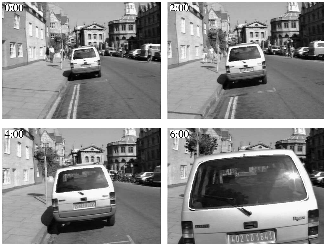
Figure 5: Using image divergence to estimate time to contact.
