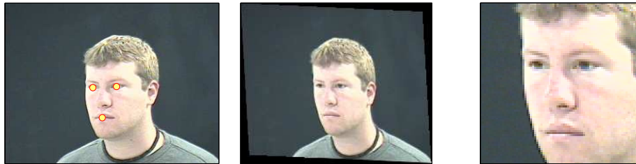
Fig. 4. Shown is the original image in the visual spectrum with detected facial features marked by yellow circles (left), the result of affine warping the image to the canonical frame (centre) and the final registered and cropped facial image.
