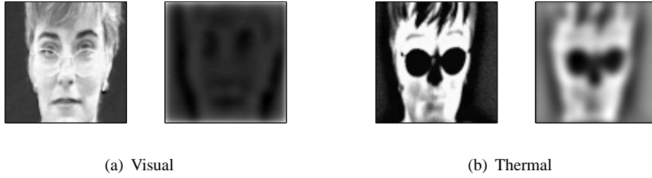
Fig. 6. Effects of the optimal band-pass filters on registered and cropped faces in (a) visual and (b) thermal spectra.
