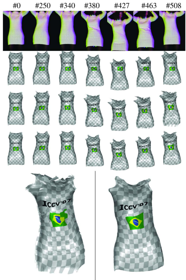
Fig. 10. Cloth tracking results of a sweater sequence. First row: Input video sequence of a person wearing a white sweater while being illuminated by three colored lights from three different orientations. Second row: Video of depth maps obtained by the technique described in Section 3 and directly texture mapped without any registration. The approach is quickly seen to fail after a few frames. Third row: Texture-mapping is obtained by advecting frame-by-frame 2D optical flow [33]. Error in the optical flow advection causes artifacts after about 380 frames. Fourth row: First method of Section 5, where 2D optical flow is regularized with a translational rigidity constraint to reduce advection errors. Last row: On the left and right, respectively, are close-ups of frame #508 taken from the third and fourth rows. Please see the video.
