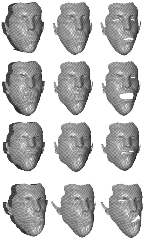
Fig. 8. Registering with different regularizations. Treating the first integrated Video Normals surface as a template that receives a checkerboard texture, we automatically register that shape throughout a long sequence by tracking flow frame-to-frame. The rows feature frames #10, #87, #116, and #290 out of 1,000. The left column uses the original translation regularization from [14], while the middle column was registered using the alternative Laplacian coordinates regularizer. Results on the right are generated like the middle column, but with the benefit of slits for the mouth and eyes, so some domain-specific input from a user.
