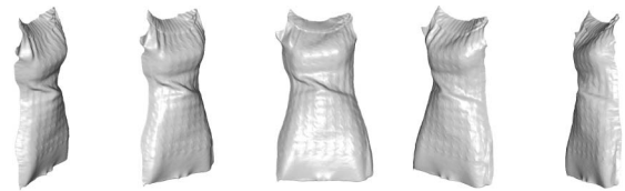
Fig. 9. Cloth reconstruction results of a deforming sweater. Multispectral photometric reconstruction of a single frame of a longer video sequence using the technique described in Section 3. Multiple viewing angles (frontal, \pm 25 degrees, \pm 50 degrees) of frame #380 of the sweater sequence. This frame is representative of the detail quality in our reconstructions for this and other tested videos.
