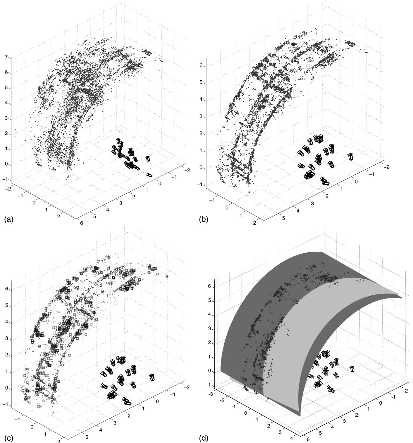
**Fig. 16.** Process of robust surface estimation: (a) reconstructed model before applying the bundle adjustment algorithm; (b) model after applying the BA algorithm; (c) classification of 3D points by SVM, surface points as rectangular markers and nonsurface points as dot markers; (d) estimation of surface, the light grey surface represents estimation with all 3D points having the weights equal to 1, and the dark grey surface is a more accurate estimation by using the weights obtained from SVM
