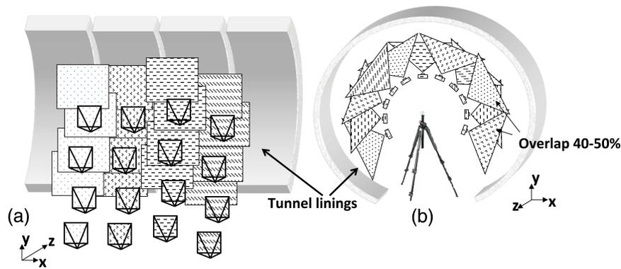
**Fig. 6.** Configuration of image acquisition system: (a) side view where the tunnel linings are in front of the camera; (b) view looking into the tunnel
