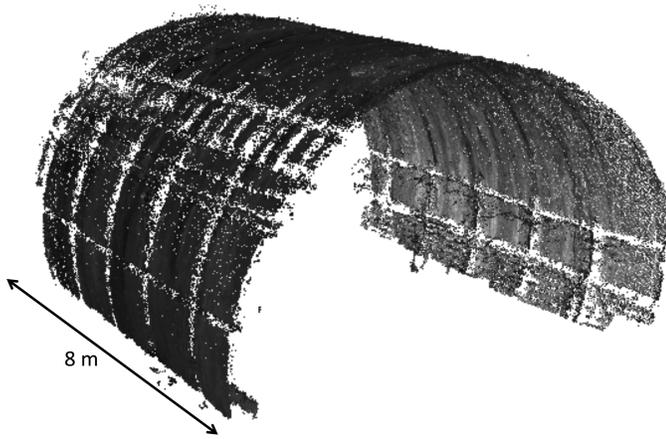
**Fig. 8.** Example of a 3D point cloud obtained from the Prague data set
