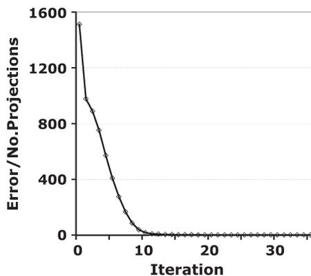
**Fig. 15.** Reprojection error of the initialized point cloud is converged when the bundle adjustment is applied
