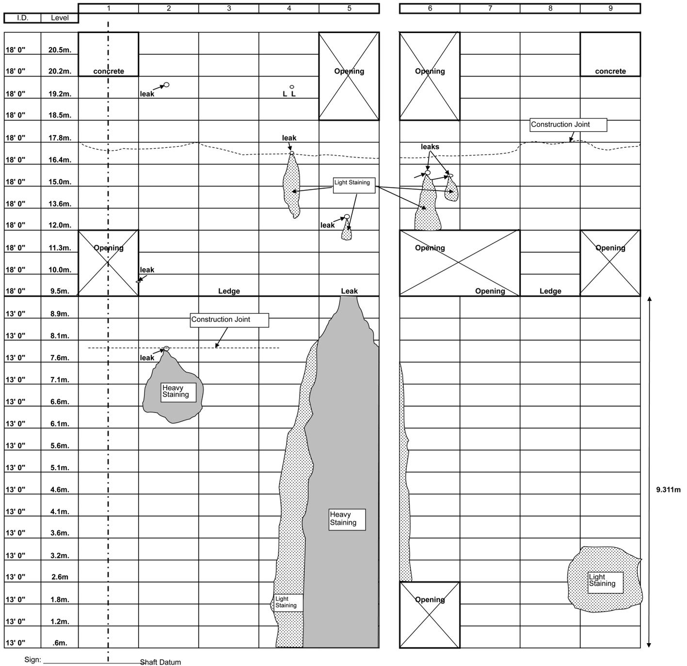
**Fig. 3.** Example of an inspection report containing sketches of anomalies on tunnel surface
