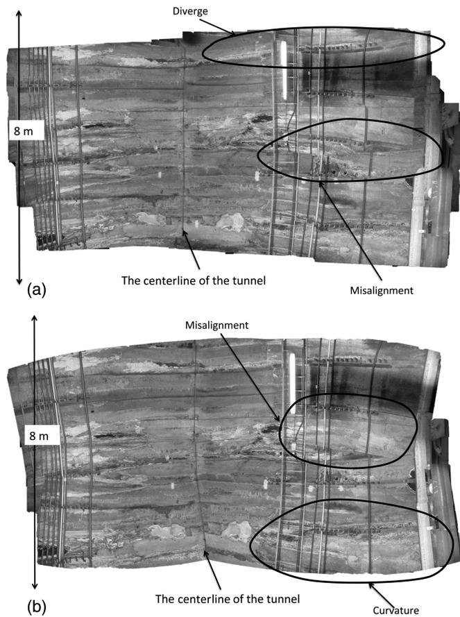
**Fig. 1.** Distortions observed in the mosaics created from typical motion models from the Prague data set: (a) homography-based mosaicing; (b) cylindrical projection mosaicing
