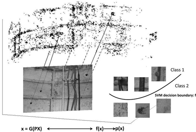
**Fig. 9.** Weights obtained from the SVM classifier are placed on 3D points for accurate surface estimation; 3D points are projected onto images by projection matrixes and then classified by the SVM classifier by their associated image points
