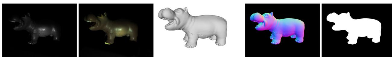
**Fig. 7** Demonstration of the processing steps performed per object in LUCES dataset. Firstly, compensation for radial distortion and demosaicing is performed on raw images to get RGB ones (left). CT-scanned
