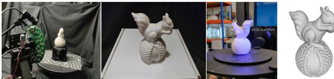
**Fig. 2** From left to right: (1) the stage of our Photometric Stereo setup, (2) a top view of a sample object (Squirrel), (3) acquisition with the GOM scanner, (4) the 3D scanned mesh
