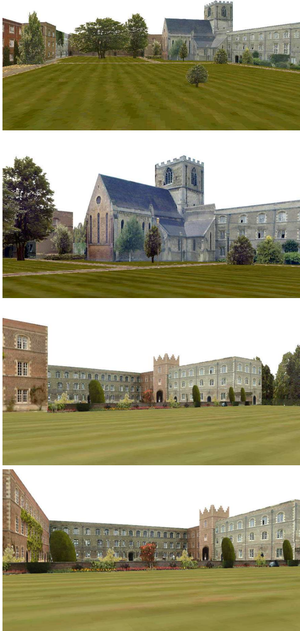
Figure 14.11: Some views of a large model of Jesus College, Cambridge. This model was reconstructed using around 50 photographs obtained using a camera with fixed but unknown focal length. The buildings in Jesus have differing orientations and so a plan of the college was used for camera calibration.
