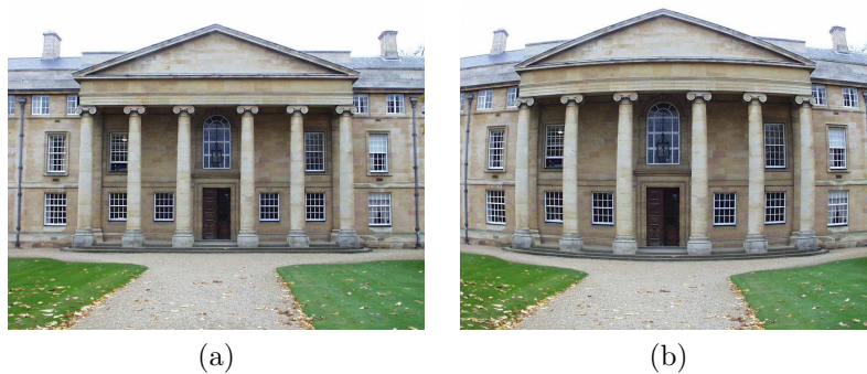
Figure 13.2: Radial distortion illustration. (a) Distortion-free image. (b) Under radial distortion, image points are displaced radially from the image centre.
