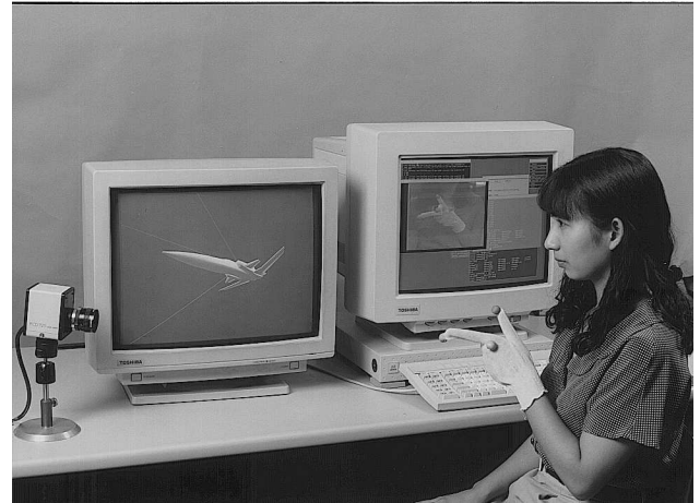
Figure 2: Vision interface using 3D hand gestures and a wireless glove.
