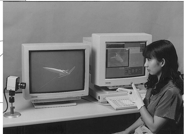
Figure 2: Vision interface using 3D hand gestures and a wireless glove.
