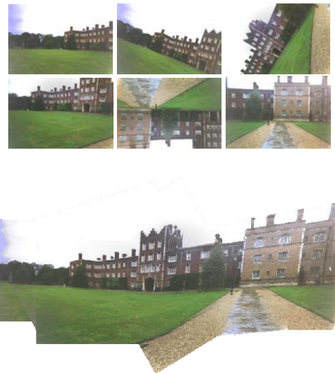
Figure 4: Result 1: A mosaic of 6 images taken with a disposable camera. The original images are shown at the top row.
