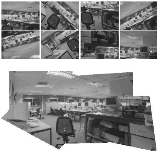
Figure 6: Result 3: A mosaic of 8 images taken with a digital camera. The original images are shown in the top 2 rows.
