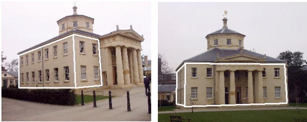
Figure 4: Original pair of photographs taken with different camera zoom setting. Six edges in each image are used to obtain the camera intrinsic parameters and the orientation and position of the viewpoints.
