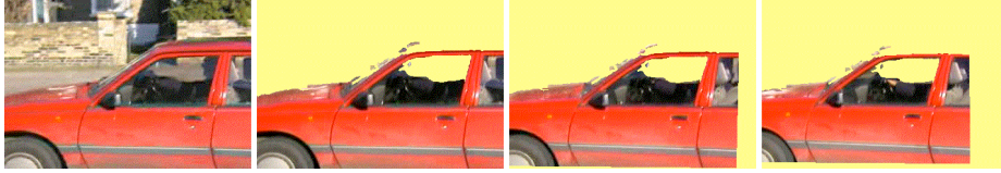
Fig. 6. Multiple-frame segmentation of the ‘car’ sequence. The camera pans to the left to track the car. Shown is the original frame 490 and then the foreground segmentation of part of the sequence, showing every 5th frame. The final region labelling is used to segment all frames in a second pass of the data.
