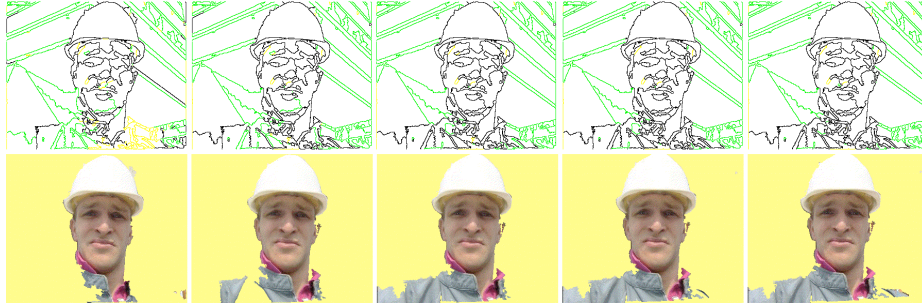
Fig. 4. Evolution of the ‘foreman’ segmentation, showing the edge probabilities and segmentations of frames 47–52 as the evidence is accumulated. The edge probabilities become more certain and small errors are removed, resulting in an improved region segmentation.
