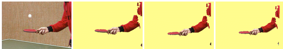
Fig. 5. Multiple-frame segmentation of the ‘tennis’ sequence. The camera zooms out while the arm slowly descends. Shown is the original frame 29 and then the foreground segmentation of part of the sequence, showing every 5th frame. The final region labelling is used to segment all frames in a second pass of the data.
