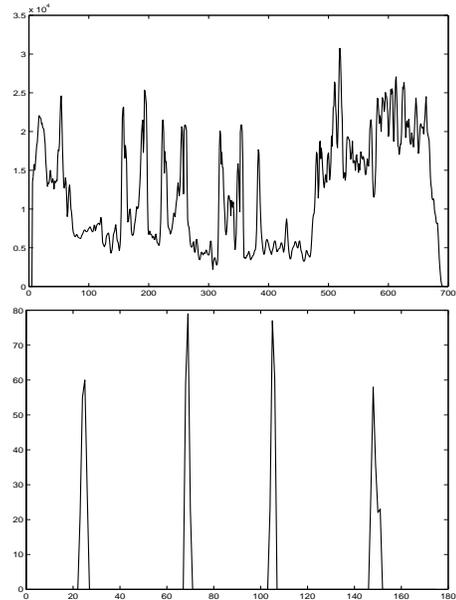
**Figure 3. Plot of the column sum of the derivative (left) and the template (right).**
