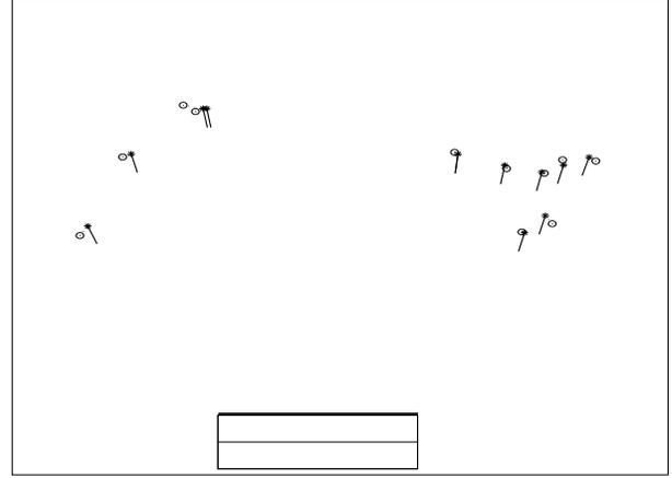
**Figure 6. The pose estimation from the matches in Figure 5 (asterisk) compared to a reconstruction based on manually estimated point correspondences (circles)**
