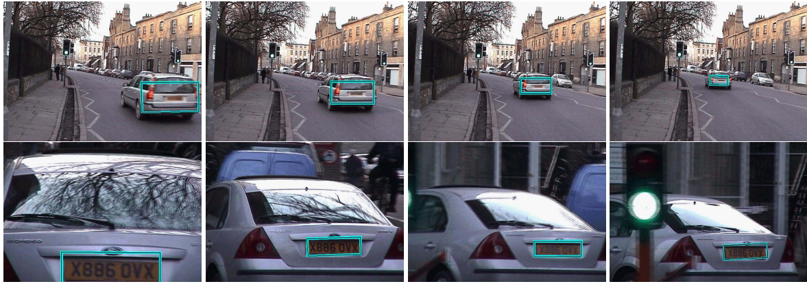
Figure 9. Tracking cars Digital video recordings of a passing vehicle and a license plate. The tracker was trained from a single frame and successfully follows the regions despite clutter and an unsteady camera.
