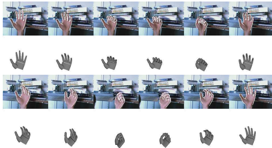
Fig. 8. Tracking a hand opening and closing with rigid body motion. This sequence is challenging because the hand undergoes translation and rotation while opening and closing the fingers. 6 DOF for rigid body motion plus 2 DOF using manifolds for finger flexion and extension are tracked successfully with our tree-based algorithm.
