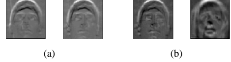
Figure 1: First two principal vectors for a comparison of two linear subspaces corresponding to the same (a) and different individuals (b). In the former case, the most similar modes of variation, represented by the principal vectors, are very much alike in spite of different illumination conditions used in data acquisition.
