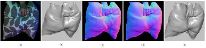
Figure 1. **Reconstruction overview**. (a) Input image. (b) Low-resolution geometry recovered from two-view stereo. (c) The normal map estimated using a constant chromaticity assumption contains large errors. (d) The normal map estimated using the proposed approach removes these errors. (e) Final high quality geometry obtained by combining stereo reconstruction with normal map.
