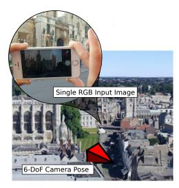
Figure 1: **PoseNet** [22] is trained end-to-end to estimate the camera's six degree of freedom pose from a single monocular image. In this paper we show how to apply a principled loss function based on the scene's geometry to learn camera pose without any hyper-parameters.
